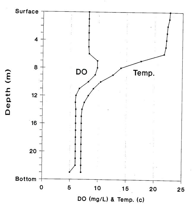
Table 21.LWQA dissolved oxygen/temperature profilesduring summer thermal stratification for SpiritLake on July 30, 1991.
