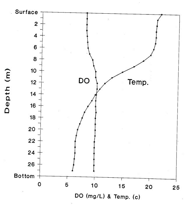
Table 10.Dissolved oxygen/temperatureprofiles during summer thermal stratificationfor Priest Lake (South) on August 2, 1991.
