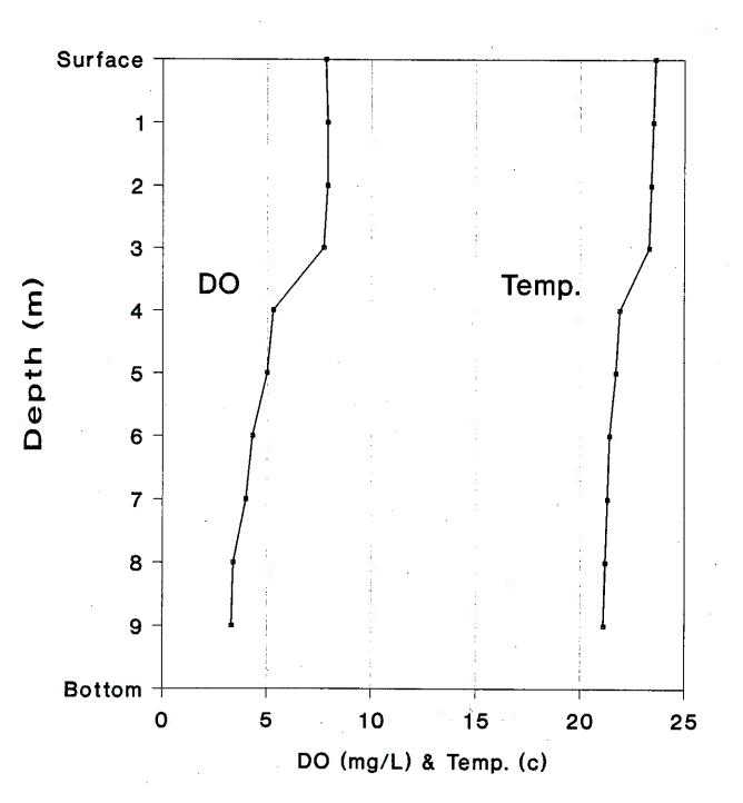
Table 60. LWQA dissolved oxygen/temperature profiles, specific conductivity and pH during summer thermal stratification for Mann Lake on August 21, 1991.
