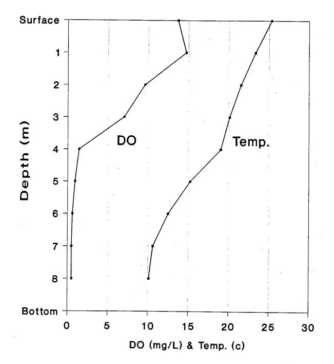
Table 62. LWQA dissolved oxygen/temperature profiles, specific conductivity and pH during summer thermal stratification for Winchester Lake on August 19, 1991.
